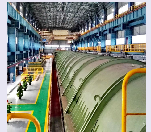
Demonstration of patent application: Flue gas circulating pre-reduction sintering process Sintering machine project, 600 square meters, Baosteel No.2 Main Plant
